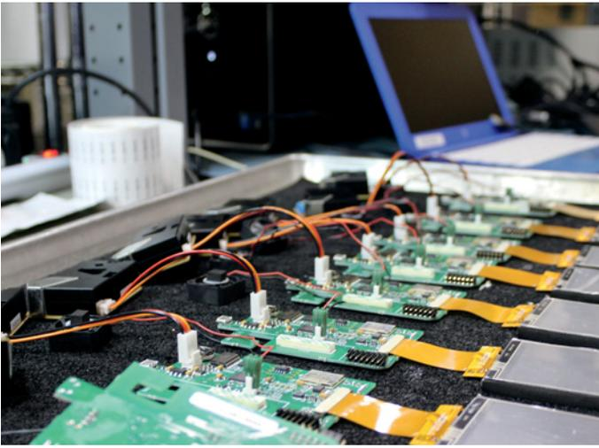
The monitor consists of a circuit board, fan and infrared sensor, among other parts. The fan creates a vacuum, drawing air past the infrared sensor. As particles pass the sensor and disrupt the beam, the chip captures each disruption, and converts those disruptions into readings that correspond roughly to the U.S. Environmental Protection Agency index for air quality. For many users, the Speck is their first glimpse at indoor air quality.
